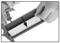
Figure 4. Loading nails into magazine.
